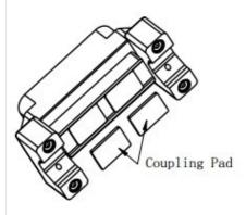
**Step 3**. Place the two base brackets directly under the upper brackets across the pipe. Finally, tighten the screws on both ends.
