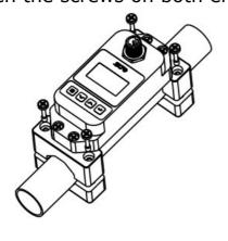
**Step 2.** Place the flow meter with the upper brackets (installed together ex-works) on the pipe. Install the meter on the side of the pipe instead of the top to avoid bubbles effecting the measurement.
