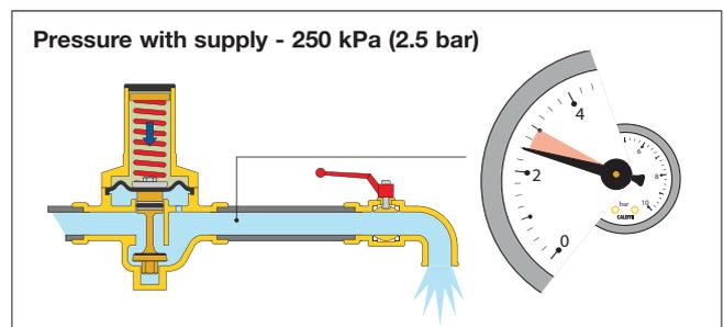
The pressure drop at the design flow rate must always be taken into account when choosing the pressure reducing valve. In addition to verifying the speed, it is always necessary to check that the pressure drop is not too high, otherwise a larger size or a different type of pressure reducing valve must be chosen.
