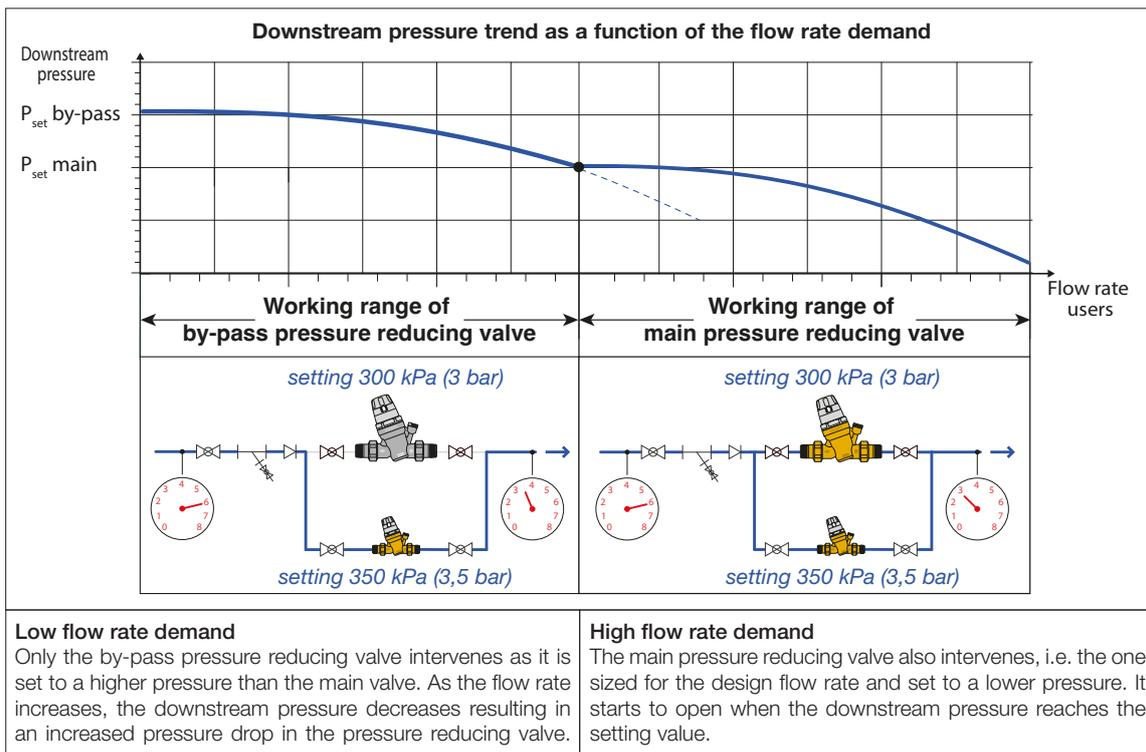
With this system solution, the pressure is fully regulated when the system is operating with a low flow rate. At the same time, the correct pressure is also guaranteed when the design flow rate is used. It is a very useful solution for systems with high flow rate demands during the day or at specific times, and significantly lower flow rates at other times.
