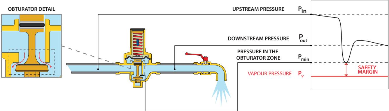
This condition causes the liquid to change to the gaseous phase, forming bubbles that contain vapour. When the bubbles implode, it causes pressure fluctuations charged with impact energy. Together with the high water speed in the gap between the seat and obturator, this can compromise the components in the pressure reducing valve, creating mechanical vibrations, noise and material erosion. The phenomenon is increased if the water contains dissolved air.
