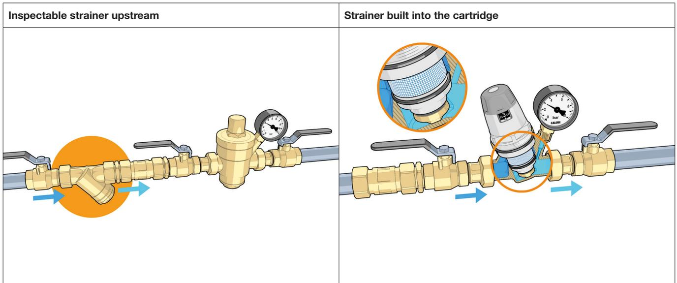
In systems with a high impurity content, it is advisable to install an inspectable strainer upstream of the pressure reducing valve, even if it already has a built-in strainer, in order to perform double filtration.
