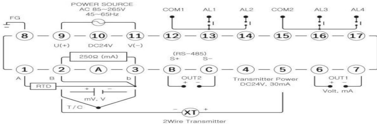
\* mA Input(+ -) Needs 250 OHM 0.05% 25ppm Resistance (2, 3 Pin)
