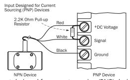
Input designed for current sourcing (PNP) devices
