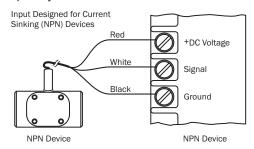
Input designed for current sinking devices (NPN)
